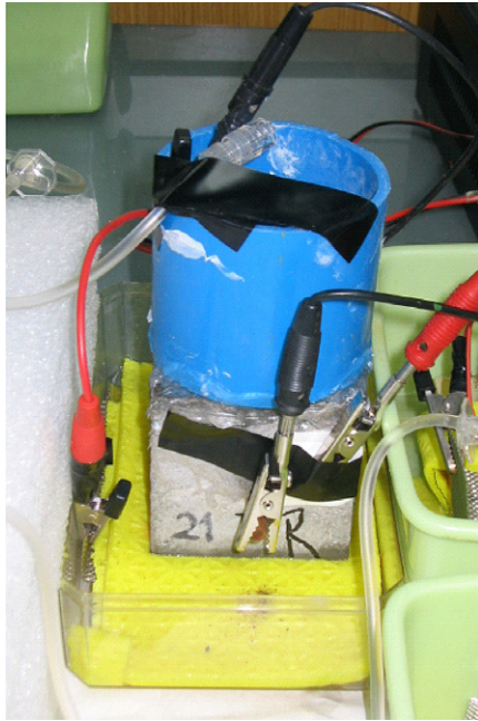
Fig. 17. Experimental arrangement used for the chloride threshold value tests.
